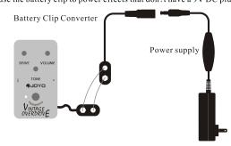
3. You can use the 3.5mm adapter to power effects that use this connector (like the EH
